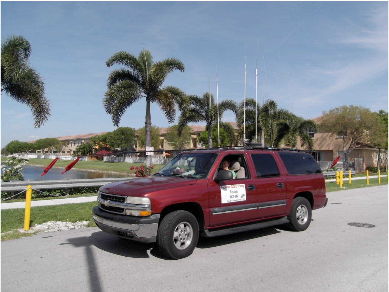
Photo 1 - Notice the fishing rods lying horizontally on the roof to extend the ground plane for the NX4N/m team
